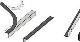
**STEP 6**From the outside of the cellar, secure the two brackets to the corresponding side of the cooling unit on exterior side of the cellar.
