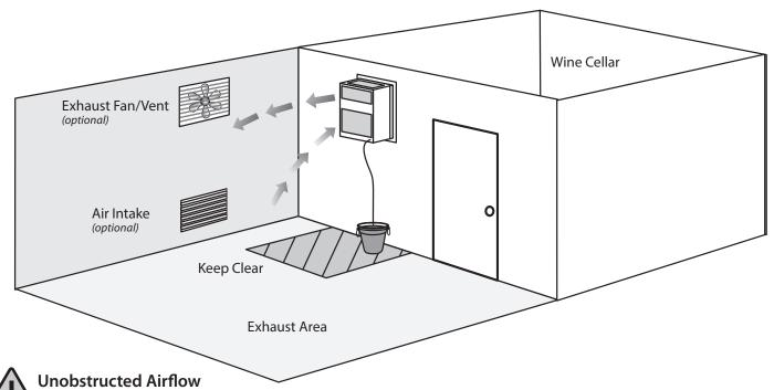
Unobstructed airflow to and from the unit is critical for the unit's overall performance and lifespan. Make sure there is a minimum of three (3) feet of horizontal clearance in every direction around the unit (fi e feet is ideal). The air blown by the fans needs to circulate and either dissipate or absorb heat from the space. The system will operate more efficiently with a greater amount of air to exchange.
