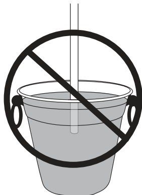
WRONG: Drain line is under water.
