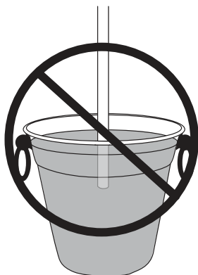
WRONG: Drain line is under water.
