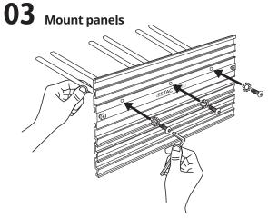
**a.** Using the hex key tightly secure the bottle supports to the panel with the included fasteners and washers.
