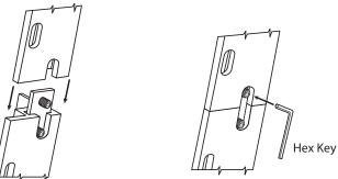
**C.** Insert coupler into second wall bracket opening.
